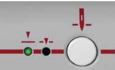
Your GrandQuilter™ will stop with the needle up or down depending on which light is switched on. After using the Thread Cutter your GrandQuilter™ will always stop with the needle in the up position.
