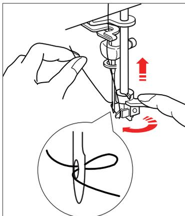
5. Turn the knob (see picture). This will draw a thread loop through the needle. Release the threader knob slowly and then pull the thread loop to the right.
