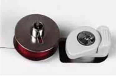
8. Cut the thread with scissors. Remove the bobbin from the bobbin winder spindle.
