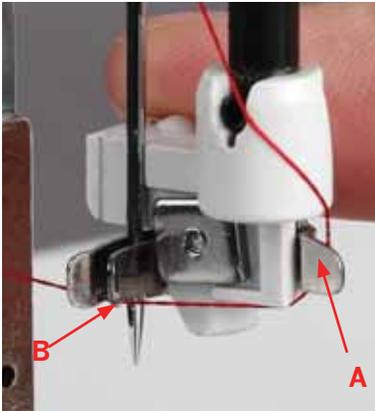
3. Pull the thread from behind around the guide (A) and under the hook (B).
