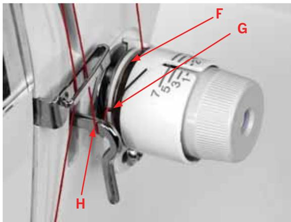
7. Draw the thread under the thread guide (H) and through the second thread guide (I). Pass the thread through the eye of the take-up lever (J).
